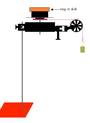
If there is very little friction on the platform, determine mathematically, in symbols, the net torque on the rotating platform containing the disk or ring. What measurements would you have to make to calculate the net torque? Show your work.
